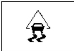
The StabiliTrak<sup>®</sup> light will flash on the instrument panel cluster when the system is both on and activated.
