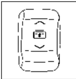
**Vent:** From the closed position, press and hold the front of the driver's side switch to vent the sunroof. Press and hold the rear of the driver's side switch to close the sunroof.
