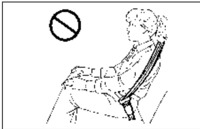
Wherever the child sits, the lap portion of the belt should be worn low and snug on the hips, just touching the child's thighs. This applies belt force to the child's pelvic bones in a crash.
