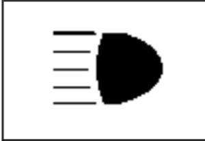
This light on the instrument panel cluster comes on if the high beam lamps are turned on while the ignition is on.
