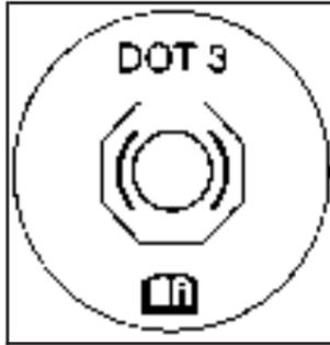
The brake master cylinder reservoir is filled with DOT-3 brake fluid. See *Engine Compartment Overview on page 396* for the location of the reservoir.
