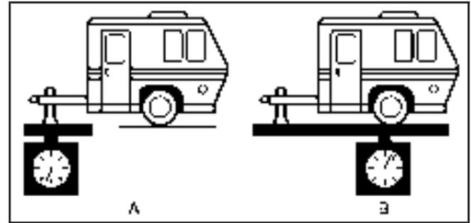
If you're using a weight-carrying hitch or a weight-distributing hitch, the trailer tongue (A) should weigh 10-15 percent of the total loaded trailer weight (B).
