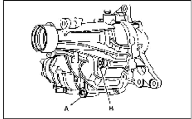
(A) Drain Plug (B) Filler Plug
