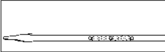
If the oil is below the cross-hatched area at the tip of the dipstick, you need to add at least one quart/liter of oil. But you must use the right kind. This section explains what kind of oil to use. For engine oil crankcase capacity, see *Capacities and Specifications on page 497*.
