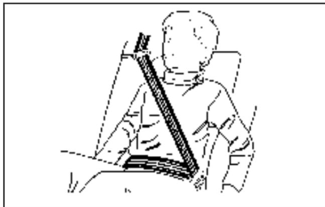
4. Buckle, position, and release the safety belt as described in *Rear Seat Passengers* on page 40. Make sure that the shoulder belt crosses the shoulder.
