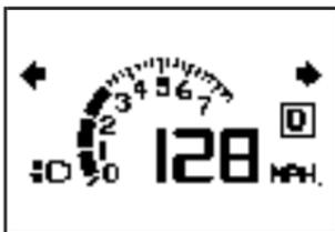
**Format Three:** This display includes all the information in Format One along with a circular tachometer, but without outside air temperature.
