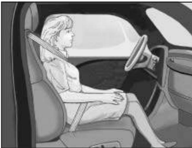
Safety belts help keep the passenger in position on the seat during vehicle maneuvers and braking, which helps the passenger sensing system maintain the passenger airbag status. See “Safety Belts” and “Child Restraints” in the Index for additional information about the importance of proper restraint use.
