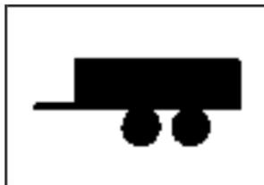
A light on the instrument panel will come on to indicate that tow/haul mode has been selected.
