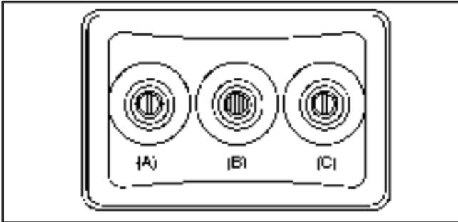
The A/V jacks located on the rear of the floor console, allow audio or video signals to be connected from an auxiliary device such as a camcorder or a video game unit to the RSE system. Adapter connectors or cables may be required to connect the auxiliary device to the A/V jacks. Refer to the manufacturer's instructions for proper usage.
