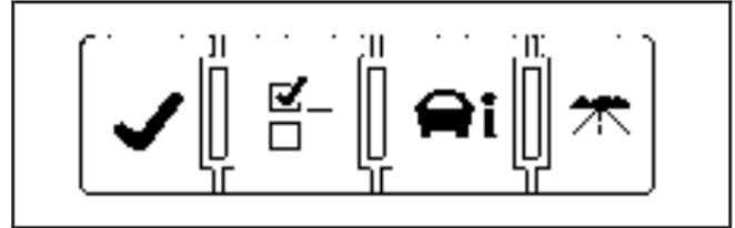
The buttons are the set/reset, customization, vehicle information, and trip/fuel buttons. The button functions are detailed in the following pages.
