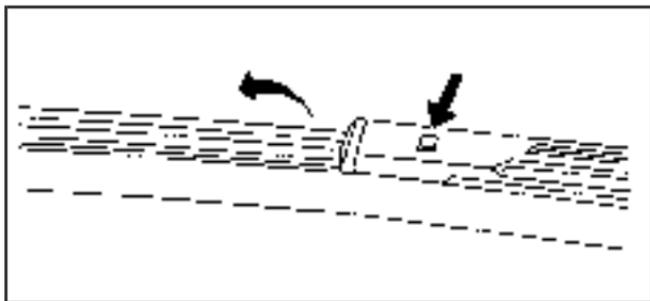
2. Press the button in the middle of the wiper arm connector, and pull the wiper blade away from the arm connector.
