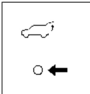
To change the liftgate to manual operation, toggle the switch on the center console to the disable position indicated by a circle.
