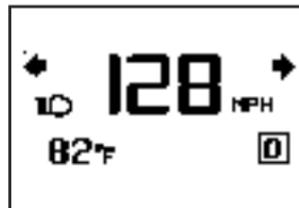
**Format One:** This display gives the speedometer reading (in English or metric units), turn signal indication, high beam indication, transmission positions, and the outside air temperature.
