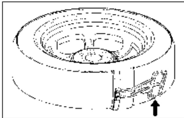
9. Remove the plastic spare tire heat shield by pulling the rubber latch. Store the plastic spare tire heat shield. See *Storing a Flat or Spare Tire and Tools* on page 472 for more information.
