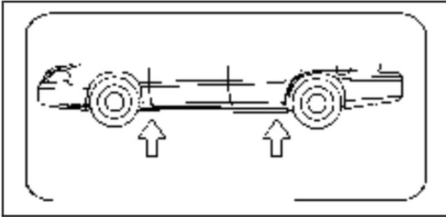
4. To identify the appropriate jacking location, find the triangle about 12 inches (30.5 cm) from the front tire or about 10.5 inches (27 cm) from the rear tire.
