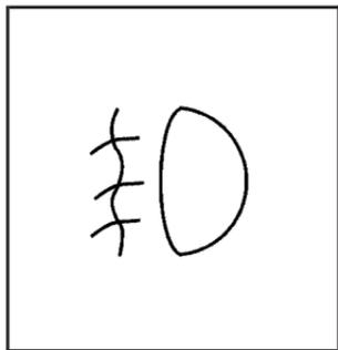
Push the button with this symbol to turn the fog lamps on or off.
