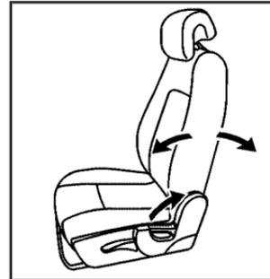
On seats with manual reclining seatbacks, the lever used to operate them is located on the outboard side of the seat.
