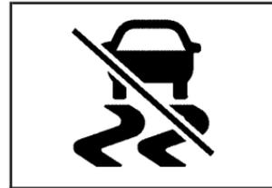
One of these TCS warning lights will be displayed on the instrument panel when the TCS is off.
