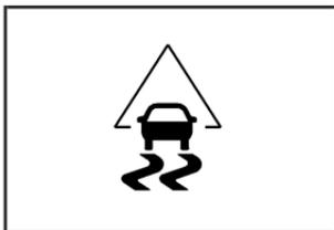
This light flashes on the instrument panel cluster while the ESC system is on and activated.
