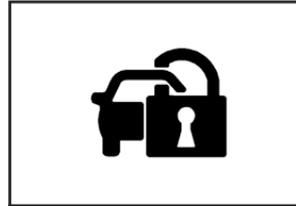
The security light, located on the instrument panel cluster, will turn on to indicate that arming has been initiated.
