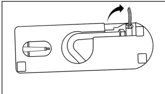
1. Unlock the air compressor inflator hose from the sealant canister by pulling the lever up.
