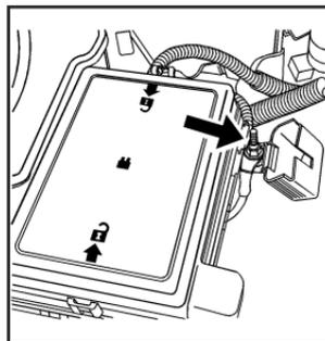
The remote positive (+) terminal is located under a red plastic cover on the engine compartment fuse block. Open the red plastic cover to access the terminal.
