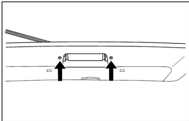
1. Remove the two screws holding the license plate lamp assembly to the fascia.
