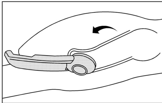
6. The convertible top front latch, located above the inside rearview mirror, must be unlatched. Pull the latch down and turn it counterclockwise to unlatch it.
