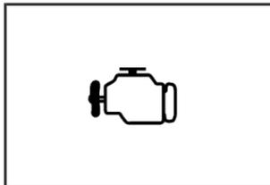
The check engine light comes on to indicate that there is an OBD II problem and service is required.
