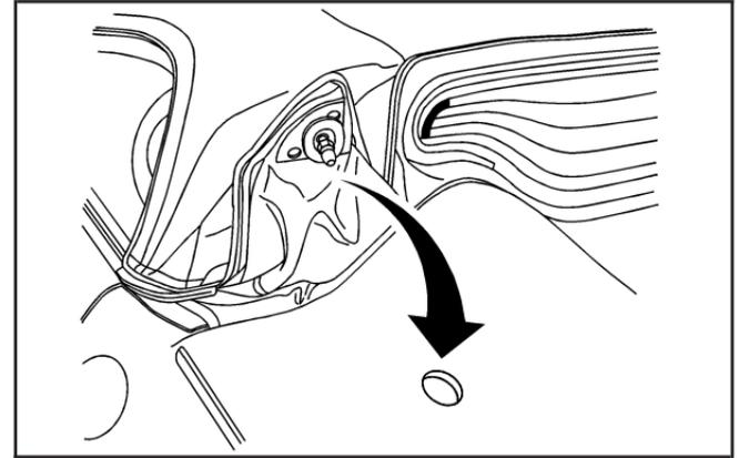
9. At the rear edge of the convertible top, press down on the two buttresses (C) to latch them into the top of the trunk.
