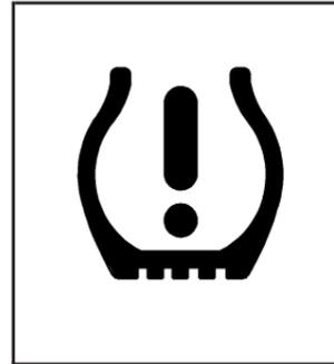
When a low tire pressure condition is detected, the TPMS turns on the low tire pressure warning light located on the instrument panel cluster.
