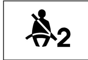
This chime and light are repeated if the passenger remains unbuckled and the vehicle is in motion.
