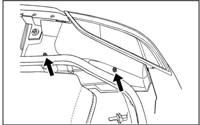
2. Remove the two screws, which hold the taillamp assembly, from inside the vehicle.
