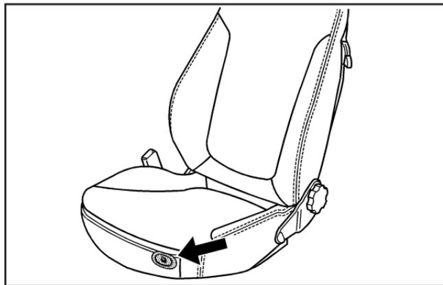
The switch is located on the front of the driver's seat on the outboard side. To use the adjuster, first move the seat to where you want it. See *Manual Seats on page 1-2*. To raise or lower the seat, hold the switch up or down.
