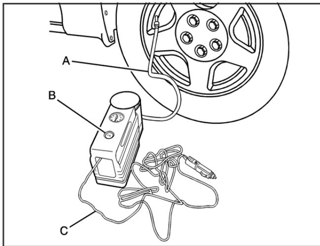
4. Attach the sealant filling hose (A) onto the tire valve stem. Turn it clockwise until it is tight.
