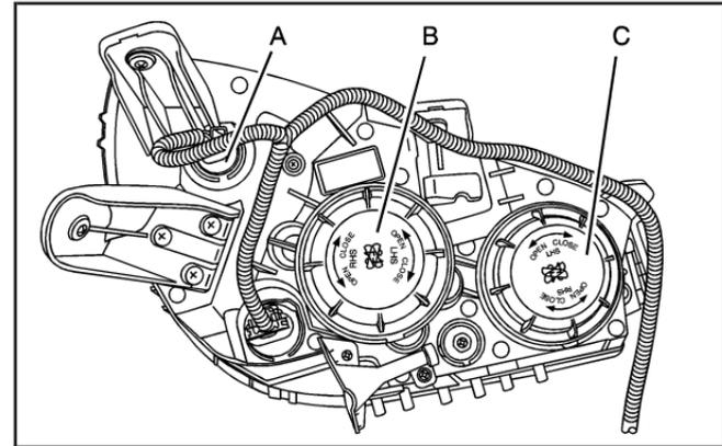
2. Remove the bulb access cover from the bulb (high or low-beam only) you need to change.
