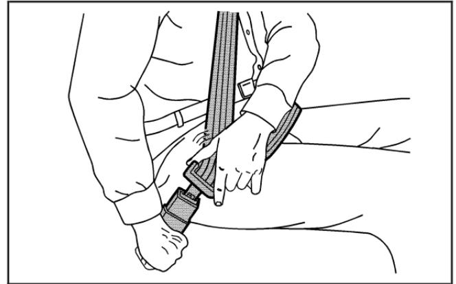
3. Push the latch plate into the buckle until it clicks. Pull up on the latch plate to make sure it is secure. If the belt is not long enough, see *Safety Belt Extender* on page 1-22.
