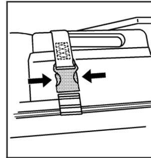
4. Remove the tire sealant and compressor kit strap by squeezing the two tabs of the quick release buckle.
