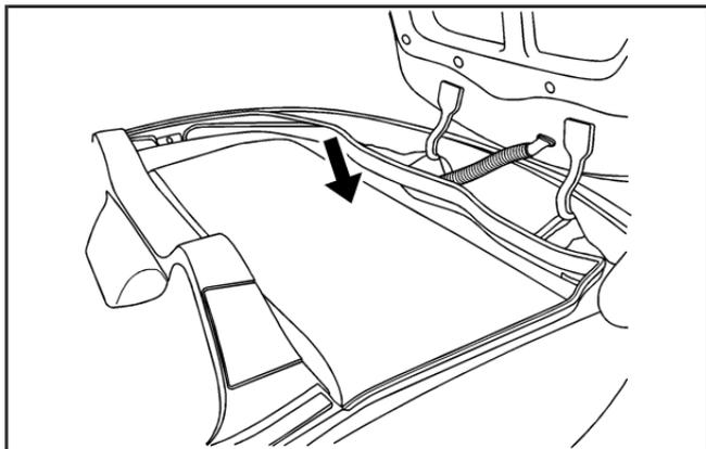
9. After the top is stored, apply one even push, as shown, on the convertible top to ensure that the top is fully retracted and securely stored.
