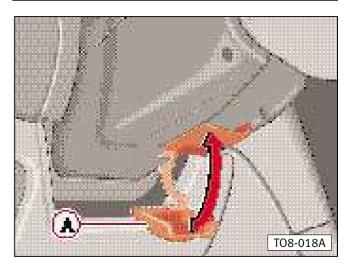
The steering column can be adjusted at will both for reach and for height. Press the lever **A** beneath the steering column down and move the steering wheel to the desired position. Then press the lever firmly up again.
