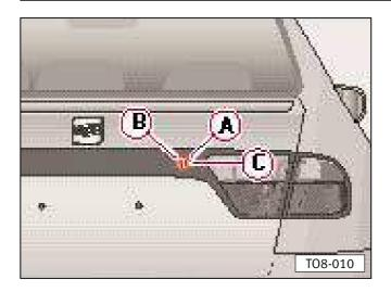
The doors can be locked and unlocked from the tailgate via the central locking system. It is also possible to lock the luggage compartment permanently
