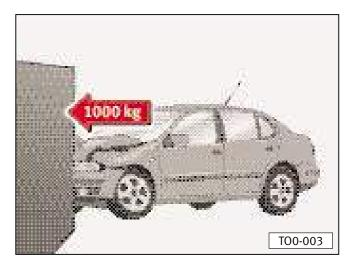
If you are driving at a speed of only 30 km/h to 50 km/h, forces which can easily exceed 1000 kg are exerted on the body should an accident occur.
