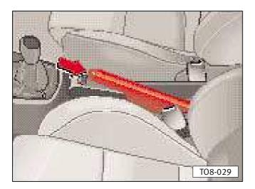
To apply the handbrake pull lever up firmly. On hills the 1st gear or with automatic gearbox the parking lock should also be engaged. The handbrake should always be applied so firmly that it is not possible to drive inadvertently with the handbrake on.
