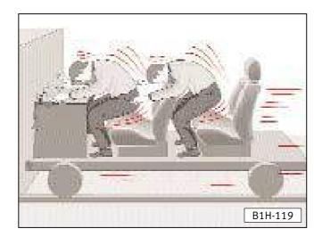
The speed of the vehicle is, however, the more important factor. If, for example, the speed increases from 25 km/h to 50 km/h, the kinetic energy increases fourfold!
