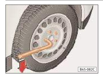
• Push the wheel spanner as far as possible onto the wheel bolt as shown and turn the spanner anti-clockwise. When doing this, grip the spanner as far as possible towards the lever end.
