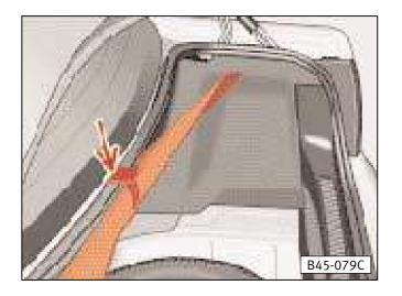
The tools are located in a polystyrene retainer, inside the spare wheel recess secured with a rubber strap.
