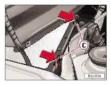
• Push back spring clips **C** in the direction of the arrow and remove the filter insert.
