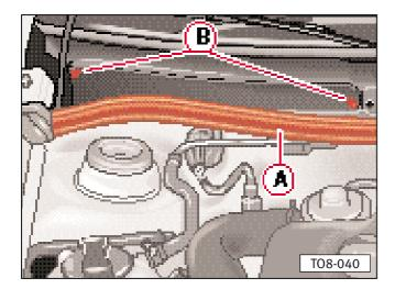
The dust and pollen filter for the heating and ventilation system can be found under the cover on the right in the plenum chamber. The filter should be changed in accordance with the details given in the Inspection and Service schedule. If the air throughput reduces considerably, the filter should be changed earlier:
