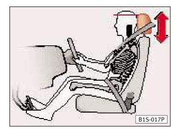
The head restraints are height adjustable and should be set to suit the size of the occupant. Correctly adjusted head restraints together with the seat belts offer effective protection. The front head restraints can also be adjusted to a different angle.
