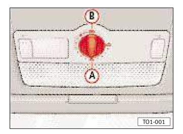
With ignition switched on, the sliding/ tilting roof can be opened and closed/ lifted and lowered with the rotary switch. Press the switch for emergency or full strength closing.
