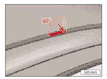
Press forcefully on the cover on the marked side in the direction of the arrow. Lift the aforementioned cover until there is a 90° angle in relation to the roof of the vehicle.
