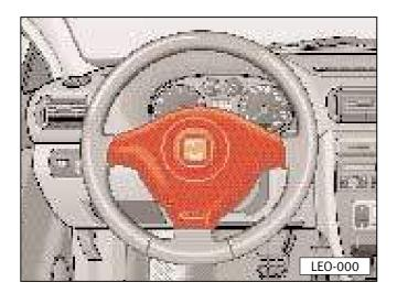
Supplementing the three-point seat belts, the Air Bag system offers additional protection for the driver's and passenger's head and chest in a serious frontal collision.
