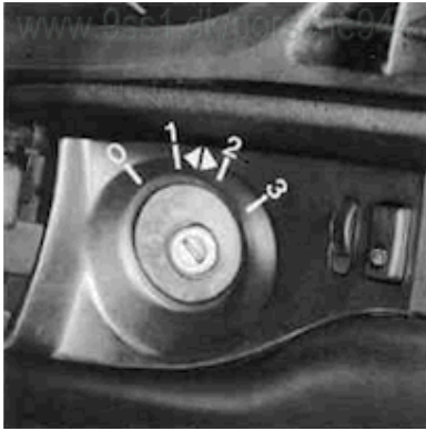
Ignition/Starter Switch with Steering Lock
