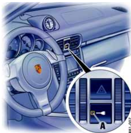
A - Light-emitting diode for alarm system
