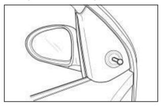
Adjust the outside manual mirrors using the control lever located next to the mirror.
