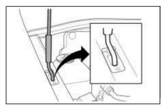
4. Place the hood prop into the slot on the inner fender.
