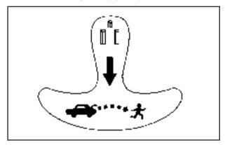
There is a glow-in-the-dark emergency trunk release handle located on the underside of the trunk. This handle will glow following exposure to light. Pull the release handle down to open the trunk from the inside.
