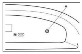
The security light (A) will flash once every second to indicate that the theft-deterrent system is armed. The security light is located on the secondary information center (SIC) on the center of the instrument panel. To avoid activating the alarm by accident, do one of the following:
