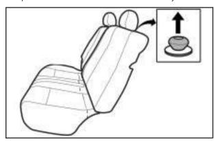
Pull up the release knob located on top of the rear seatback.
