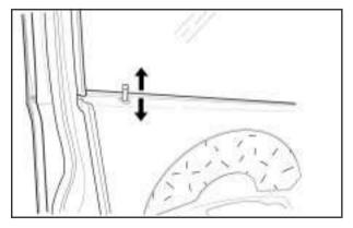
From the inside, you can lock and unlock all of the doors by pushing or pulling the manual door lock located on the window sill on each door.
