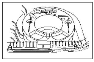
Remove the foam tray from the cargo area. Remove the jack, the jack handle and the wheel wrench from the foam tray. The jack is stored in the front center area of the foam tray.
