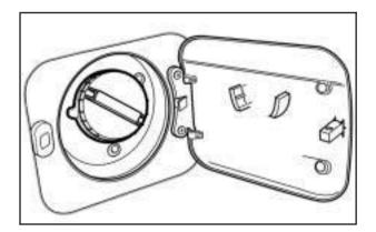
The tethered fuel cap is located behind a hinged door on the passenger's side of your vehicle.
