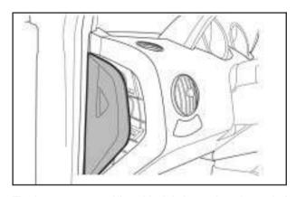
The instrument panel fuse block is located on the end of the instrument panel on the driver's side of the vehicle. To access the fuses, open the fuse panel door by pulling the door out.
