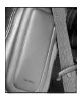
If your vehicle has a side impact air bag for the driver it will say AIR BAG on the air bag covering on the side of the driver's seatback closest to the door
