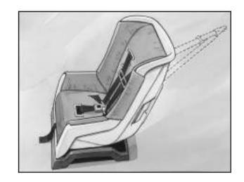
In Canada, the law requires that forward-facing child restraints have a top strap, and that the strap be anchored. In the United States, some child restraints also have a top strap. If your child restraint has a top strap, it should be anchored.
