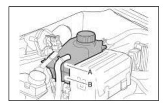
The coolant level should be between the MIN (B) and MAX (A) marks on the coolant surge tank when the engine is cool. If it is not, you may have a leak at the pressure cap or in the radiator hoses, heater hoses, radiator, water pump or somewhere else in the cooling system.
