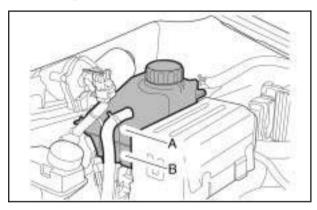
The engine coolant surge tank is located in the rear of the engine compartment on the driver's side. See *Engine Compartment Overview on page 5-14* for more information on location.
