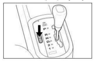
Press the HOLD button on the shift lever console to turn on hold mode. Press the button again to turn off hold mode, and return to normal automatic transaxle operation. While on, the HOLD indicator light on the secondary information center will light up. See *Hold Mode Light on page 3-28*.
