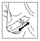
The tilt wheel lever is located underneath the steering column slightly to the left.
