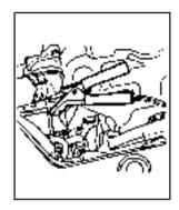
9. Connect the other end of the negative (–) cable at least 18 inches (45 cm) away from the dead battery, but not near engine parts that move. The electrical connection is just as good there, and the chance of sparks getting back to the battery is much less.
