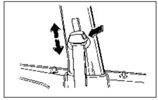
To move the shoulder belt height adjuster down, squeeze the release button and move the height adjuster to the desired position. You can move the height adjuster up just by pushing up on the shoulder belt guide. After you move the adjuster to where you want it, try to move it down without squeezing the release button to make sure it has locked into position.
