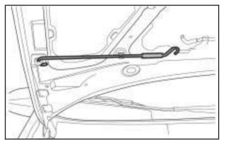
3. Lift the hood and release the hood prop from its retainer located on the underside of the hood.
