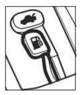
Open the trunk on your sedan from inside your vehicle by pulling up the release lever located to the left side of the driver's seat.
