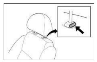
Push in the release button and press down on the head restraint in order to adjust the position downward.
