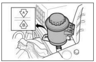
The level should be between the MIN (B) and MAX (A) marks on the reservoir. If the level drops below the MIN (B) mark, add the power steering fluid.
