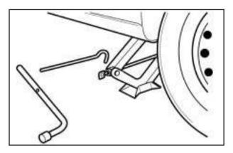
4. Insert the jack handle into the jack and the wheel wrench onto the end of the jack handle.
