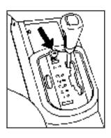
Insert the key into the shift-lock release slot and press and hold the key.
