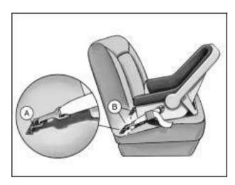
In order to use the LATCH system in your vehicle, you need a child restraint designed for that system.
