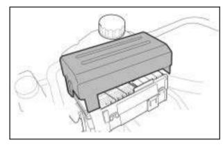
The engine compartment fuse block is located on the driver's side of the vehicle, near the battery. See *Engine Compartment Overview on page 5-14* for more information on location. To access the fuses, pull out the top and bottom flaps to release the cover. To reinstall the cover, push the cover until it is secure.
