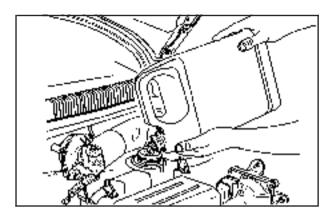
3. Fill the coolant surge tank with the proper mixture to the MAX (A) mark on the coolant surge tank. Wait about five minutes, then check to see if the level is below the MAX (A) mark. If the level is below the MAX (A) mark, add additional coolant to bring the level up to the MAX (A) mark. Repeat this procedure until the level remains constant at the MAX (A) mark for at least five minutes.
