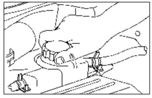
Then replace the pressure cap. Be sure the pressure cap is hand-tight and fully seated. See your dealer, if necessary.
