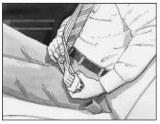
If the belt stops before it reaches the buckle, tilt the latch plate and keep pulling until you can buckle it. Pull up on the latch plate to make sure it is secure. Make sure the release button on the buckle is positioned so you would be able to unbuckle the safety belt quickly if you ever had to.
