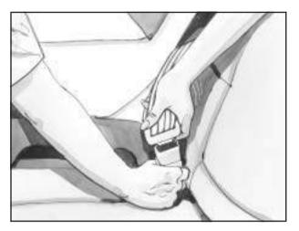
3. Buckle the belt. Be sure the latch plate clicks when you put it into the buckle. This means you are using the correct buckle. Also, make sure the release button is positioned so you would be able to unbuckle the safety belt quickly if you ever had to.
