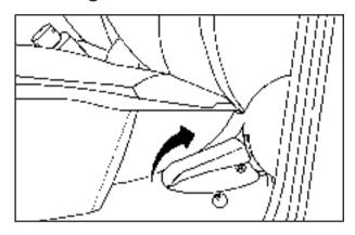
To adjust the seatback, pull up the lever located on the outboard side of the seat and move the seatback to where you want it.
