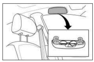
If your vehicle has this feature, the sunglasses storage compartment is located above the driver's door. To open the sunglasses storage compartment, pull down and hold the upper part of the cover. To close the compartment, let go of the cover and the compartment will automatically close.
