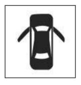
When the ignition is on, this light will stay on until all doors are closed and completely latched.
