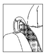
Insert the upper part of the safety belt into the safety belt guide.
