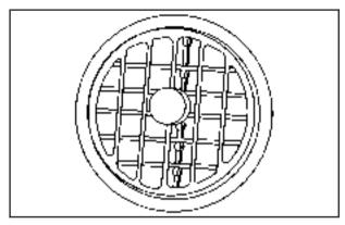
Use the knob located in the center of each outlet to change the direction of the airflow.
