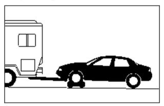
Notice: Towing your vehicle from the rear with the front wheels on the ground could cause transaxle damage. Do not tow the vehicle from the rear with the front wheels on the road.
