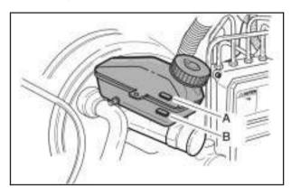
To check the fluid level, look on the side of the reservoir. If the fluid reaches the MAX (A) mark on the reservoir, the fluid level is correct. The reservoir is located near the back of the engine compartment on the driver's side of the vehicle. See *Engine Compartment Overview on page 5-14* for more information on location.
