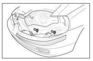
5. Turn the front turn signal bulb socket counterclockwise.
