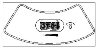
The thumbwheel for this feature is located on the instrument panel to the left of the steering column. Turn the thumbwheel to the right to brighten the lights or to the left to dim them
