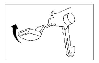
2. Then go to the front of the vehicle and push the secondary hood release lever up.
