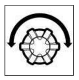
To adjust the height of the driver's seat cushion, turn the knob located on the outboard side of the seat cushion.
