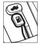
To open the fuel filler door, pull up on the fuel filler door release lever located on the floor to the left of the driver's seat
