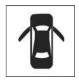
If one of the doors on your vehicle is not closed properly while the ignition is on, the door ajar light on the secondary information center will come on and stay on until the doors are closed.
