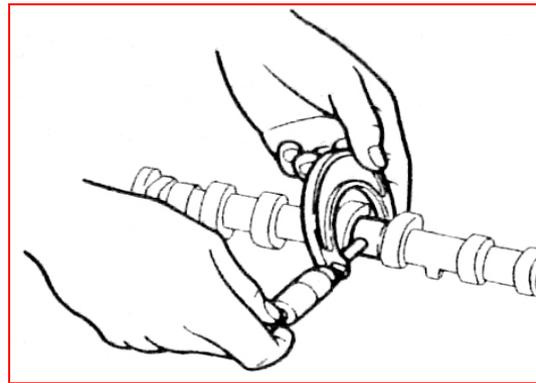
Replace with the new camshaft if the measured value exceeds the limit value.
