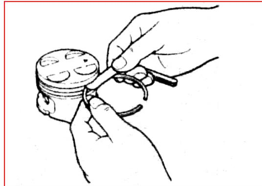
Replace with the new one if the examined clearance cannot be worn and torn any longer.
