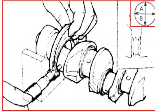
Rotate the crankshaft 90° and measure it again.
