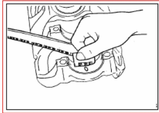
e): Dismantle the main bearing cap carefully.
