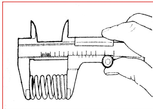
Replace with the new valve spring if the measured value exceeds the limit value.
