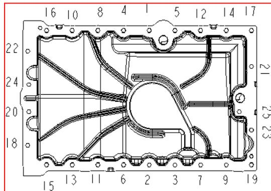
See the diagram for screwing sequence.
