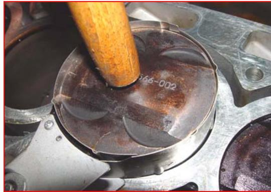
Note: the end of connecting rod with a point should face the cylinder and consists with the arrowhead on the top side of piston.
