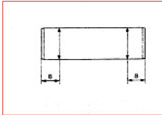
b. Measure the diameter of piston pin hole around with micrometer gauge for inside diameter, as the following picture, and take the minimum value as the diameter of pin hole.
