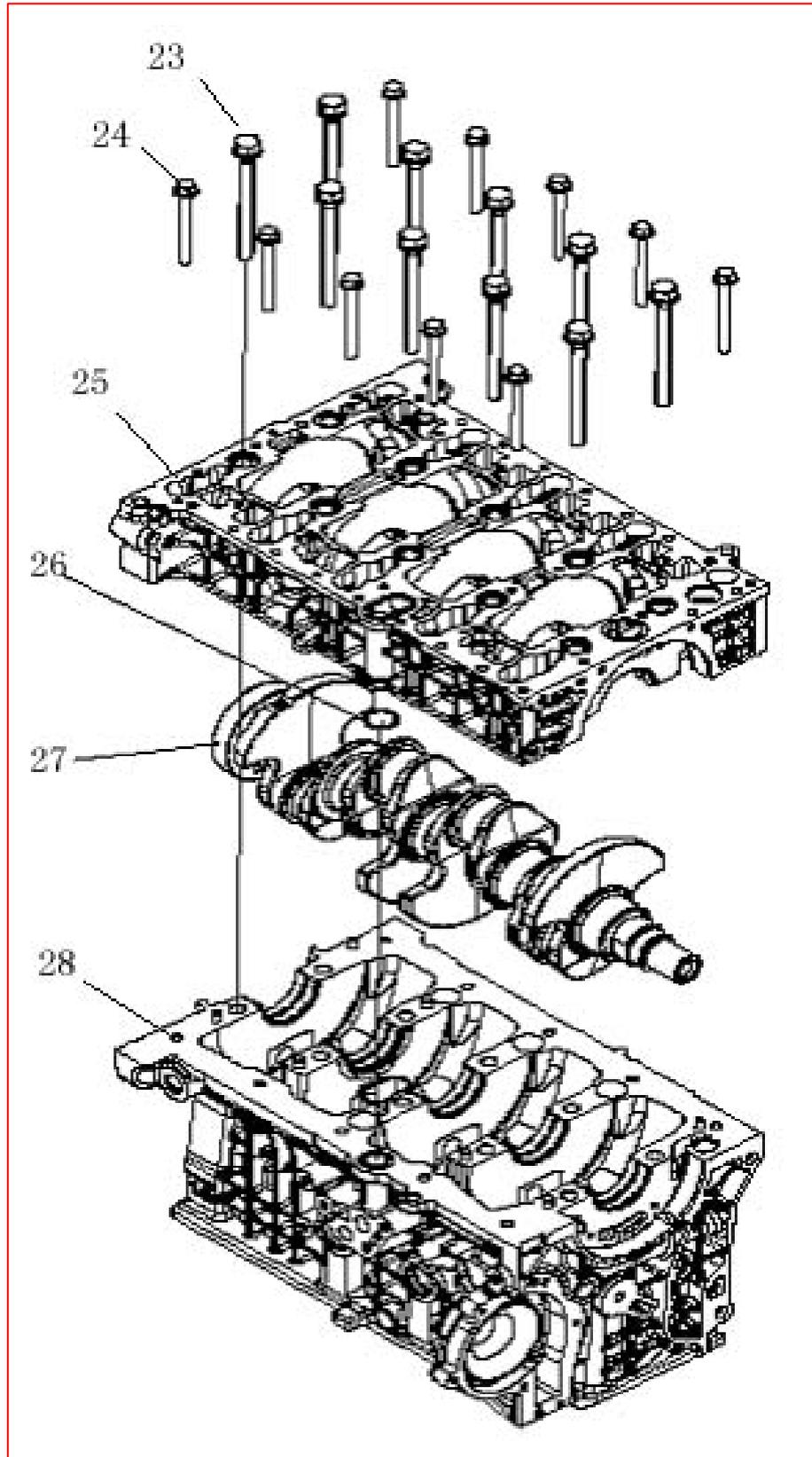
23. Crankshaft Main Bearing Bolt
