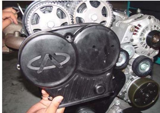
2. Remove the lower cover of engine timing belt.
