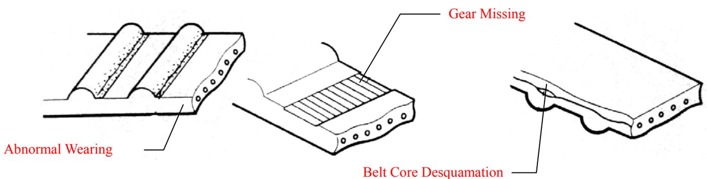
Replace the belt as any following situation occurs, even though abrasion cannot be found directly.
