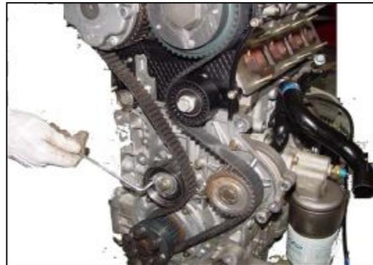
9. Lift down the special timing calibration tools, and then fasten the valve chamber cover, timing belt cover, the right engine mounting bracket of engine, and dynamo belt.
