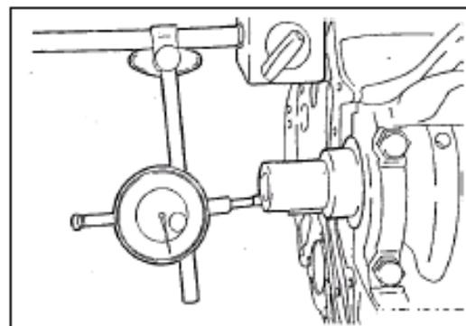
If the measured value exceeds the limit value, please replace the thrust washer.
