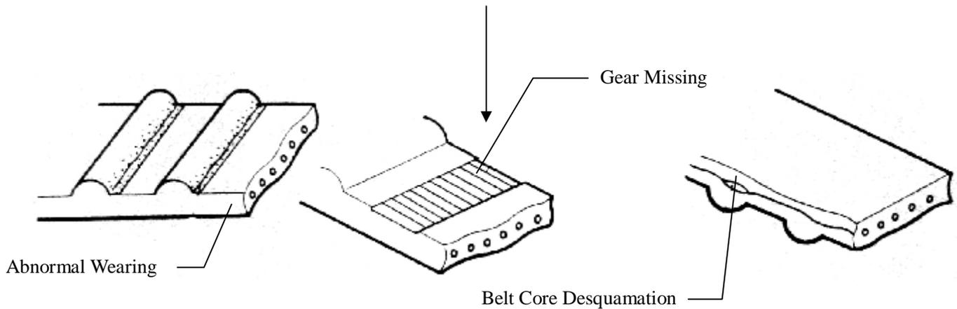
Even if no outer damage is confirmed, you should also replace the belt when any of the following conditions occurs.
