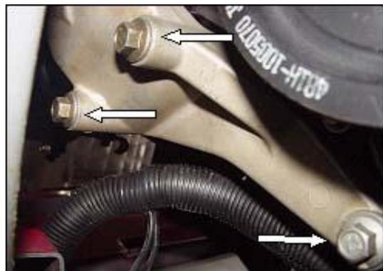
15. Loosen the three bolts of right suspension cushion, and dismantle the right suspension cushion assembly and bracket.
