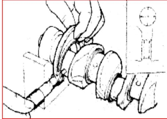
Rotate the crankshaft for 90°, and carry out measurement.
