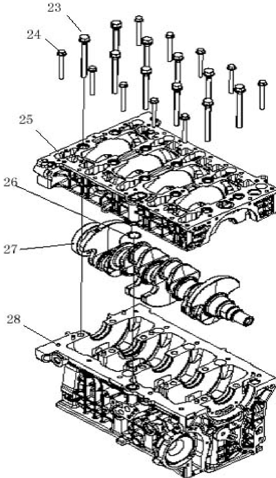
23. Crankshaft Main Bearing Bolt
