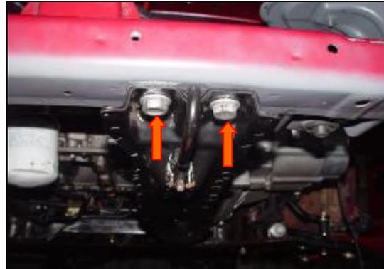
12. Remove the hexagonal flange bolts of rear suspension-cushion assembly of engine.
