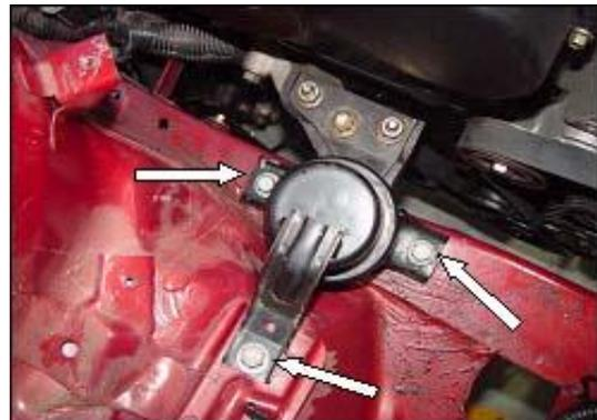
16. Dismantle the hexagonal flange bolts of left suspension cushion in order to ensure no connection between the engine and car body. Lift down the crane carefully and shift out the power assembly.
