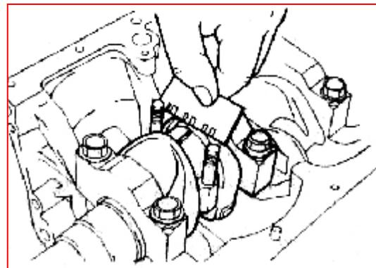
Loosen the connecting rod bolt, dismantle the bearing cap; and use the measuring rule on the clearance gauge packaging bag to measure the width of the widest portion of the flattened clearance gauge, and get the clearance value.
