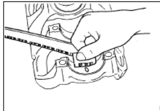
If the clearance value exceeds the limit value, please replace the bearing bushing.
