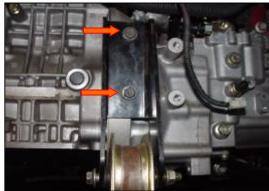
11. Dismantle the hexagonal flange bolts of girder under the car body.
