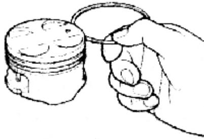
b. Use feeler gauge to measure the clearance between the piston ring and ring slot.
