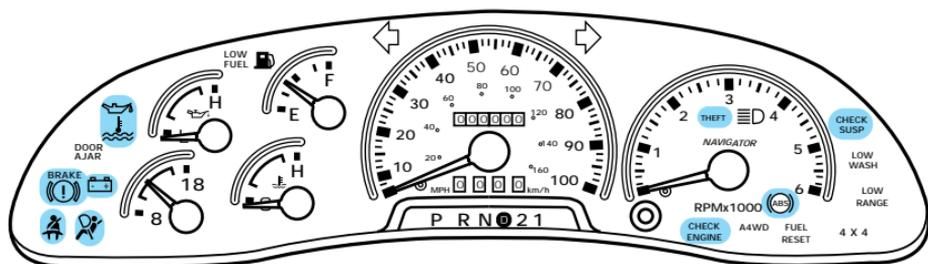
Make sure the corresponding lights illuminate briefly. If a light fails to illuminate, have the vehicle serviced.
