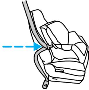
4. Insert the belt tongue into the proper buckle for that seating position until you hear and feel the latch engage. Make sure the tongue is latched securely by pulling on it.
