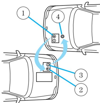
5. Make sure that the jump leads are clear of moving parts of the engine.
