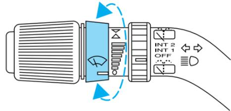
Push the control on the end of the stalk to activate washer. Push and hold for a longer wash cycle.
