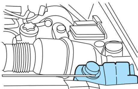
If the engine coolant has not been checked for a long period of time, the engine coolant reservoir may eventually empty. If this occurs, add engine
