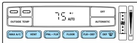
The air conditioning compressor will operate in all modes except FLOOR and VENT. It will also operate only when required when AUTOMATIC has been selected. However, the air conditioning will only function if the outside temperature is about 10°C (50°F) or above.
