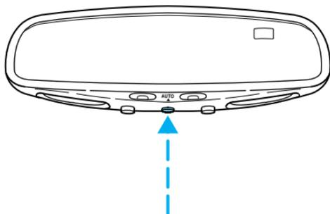
On vehicles equipped with a moonroof, the automatic rear view mirror has two map lamps. Refer to *Interior lights* for more information.
