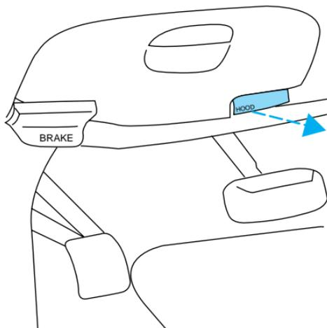
2. Go to the front of the vehicle and release the auxiliary latch located under the front of the hood, just above the passenger side headlamp. Slide the yellow handle to release the auxiliary latch.
