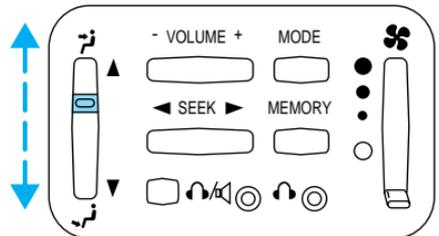
The instrument panel climate controls must be on in order for the rear climate control console controls to work.
