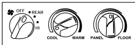
The instrument panel climate controls must be on in order for the auxiliary A/C-heater to operate.
