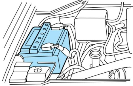
If the electrolyte level in the battery is low, you can add plain tap water to the battery, as long as you do not use hard water (water with a high alkali content). If possible, however, try to only fill the battery cells with distilled water. If the battery needs water often, have the charging system checked.
