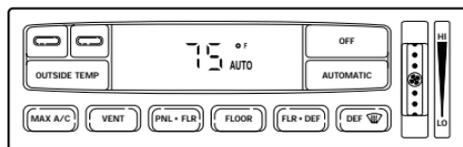
When the auxiliary A/C-heater control is set to FLOOR, airflow only occurs from the third row seat floor vent located in the driver's side rear quarter trim panel.
