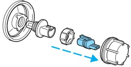
7. Remove the bulb retainer ring by turning it counterclockwise about  $\frac{1}{4}$  turn, then slide the ring off the plastic base.
