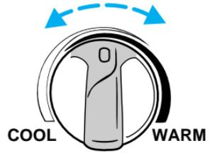
You can get warm or cool air through either the overhead registers or floor vent by turning the auxiliary mode selector:
