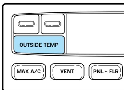
If the selected temperature is changed while the outside temperature is displayed, the new temperature will be displayed for four seconds after it is changed, then the outside temperature will return to the window.
