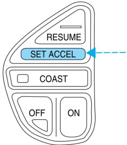
You can accelerate with the accelerator pedal at any time during speed control usage. Releasing the accelerator pedal will return your vehicle to the previously programmed set speed.
