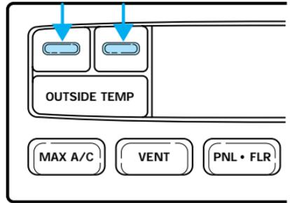
For continuous maximum cooling, push the blue button until 16°C (60°F) is shown in the display window. The EATC will continue maximum cooling (disregarding the displayed temperature) until a warmer temperature is selected by pressing the red button.
