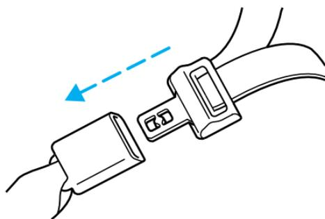
2. To unfasten, push the red release button and remove the tongue from the buckle.
